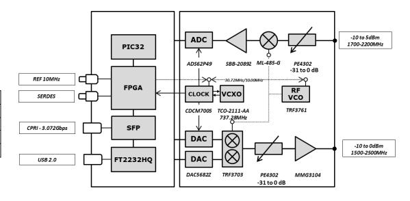
The RRU Demonstration Unit supports up to 100MHz of transmit bandwidth using a Texas Instruments DAC5682z DAC and TRF3703 mixer operating in either ZIF or CIF configurations. Receiver or DPD observation is provided by a TI ADS61B49 ADC with TriQuint ML-485 for 3G-4G-IMT or ML-483 for 4G-US-EDD variants.
