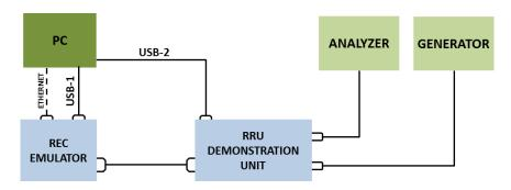
Figure 3: RRU and REC Emulator Setup for 3GPP Performance
