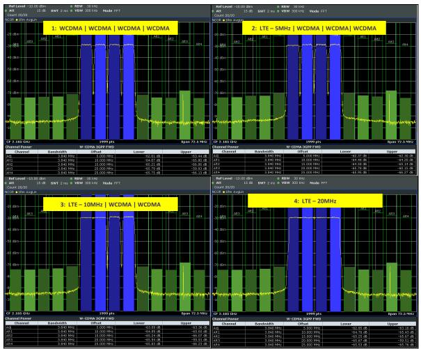
Figure 6: WCDMA + LTE Multi-Mode 3GPP Test Examples
