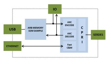
Figure 2: CPRI REC Emulator Functional Diagram
