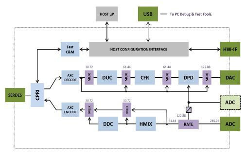
Figure 1: Demonstration RRU FPGA Functional Diagram
