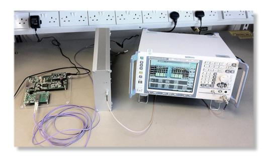
Figure 5: RRU and REC Emulator Setup for 3GPP Performance Testing
